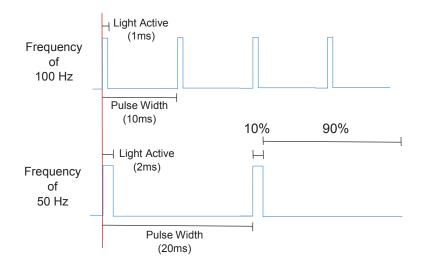
The Stroboscope will set the frequency of the pulse. The module will always operate at a 10% duty cycle.
